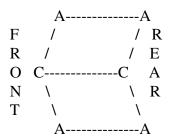
Between each A - A position (2), place one 10' Frame Pole and secure loosely
